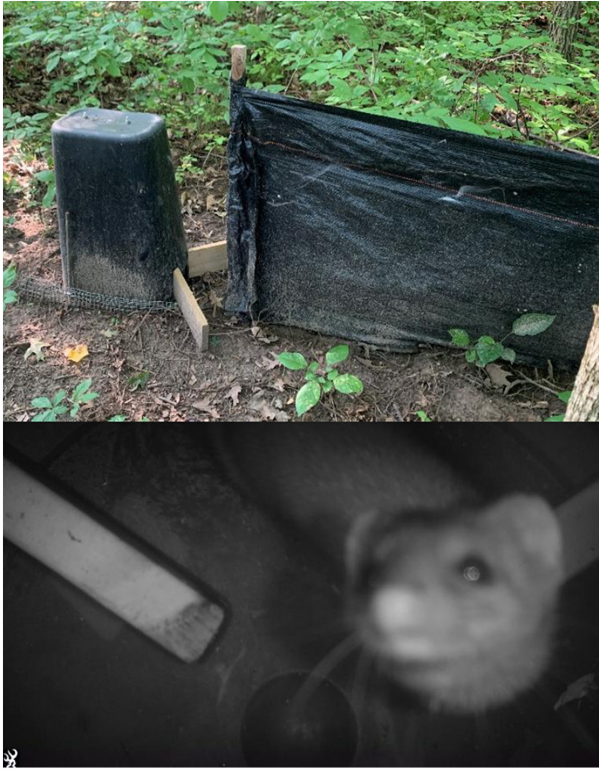
Fig. 6. Top: AHDriFT system deployment showing drift fence with modified overturned trash can at end to direct animals into the trash can. Bottom: Inside the trash can a downward facing camera takes a photo of a weasel in Indiana, USA (photo credit: Scott Bergeson and Carsten White).
